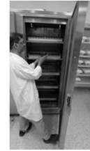
3. Cure the specimens at 35 \pm 3^\circ\text{C} ( 95 \pm 5^\circ\text{F} ) for 23 \frac{1}{2} \text{ h} \pm 30 \text{ min} . At 23 \frac{1}{2} \pm 6 \text{ 30 min} , remove molds from container and demold the specimens
