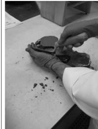
4. Draw Flat Side Trowel at Right Angle to Length of Mold.
