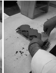
5. Draw Flat Side of Trowel Lightly Down Length of Mold.
