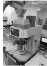
1. Mix Cement Mortar per ASTM C305. Proportions are Provided in ASTM C109.
