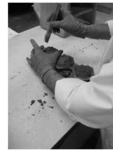
2. Mold Six Mortar Bars and Up To 21 Cubes for Compressive Strength.
